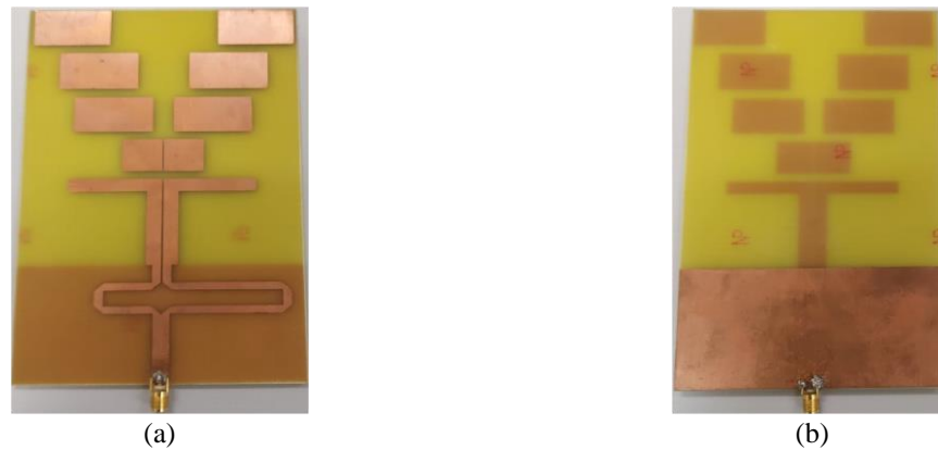
Figure 3. Fabricated prototype of the quasi-Yagi antenna (a) front view and (b) back view
