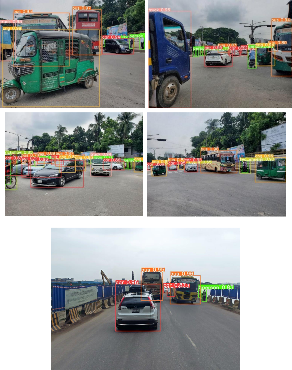
Figure 4.3.1: Test result using YOLOv8l.
