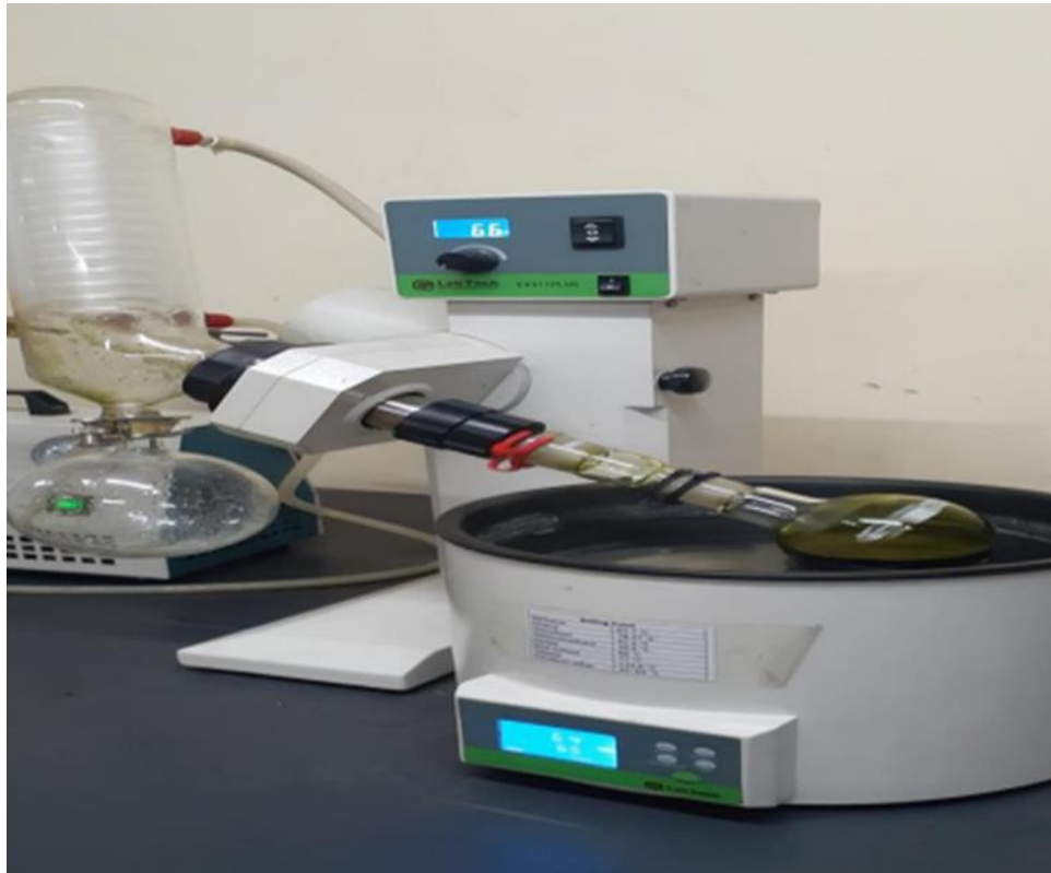
Figure 3: Evaporation of extract via Evaporator
