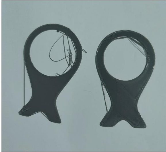
Figure 4.4: Bevel issue comparison side by side 1 st one has stringing and 2 nd one is clean
