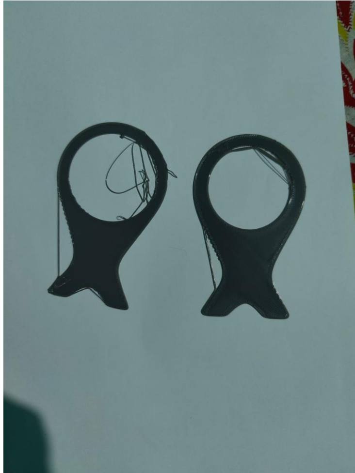
Figure 2.7: Stringing issue when we use more bevel on the model it causes stringing
