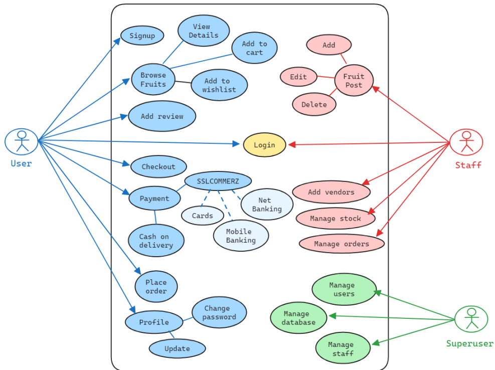
Figure 3.2.2: Use Case Diagram
