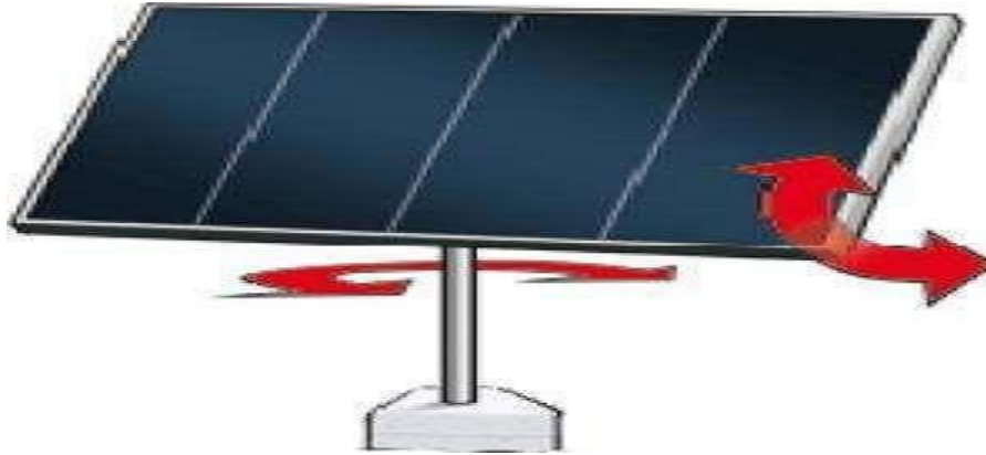
Figure 2.13: Dual-axis solar tracking
