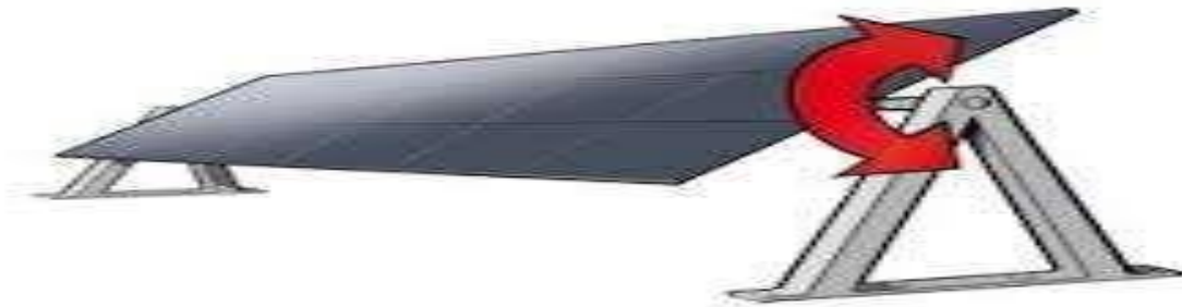
Figure 2.12: Single axis solar tracker
