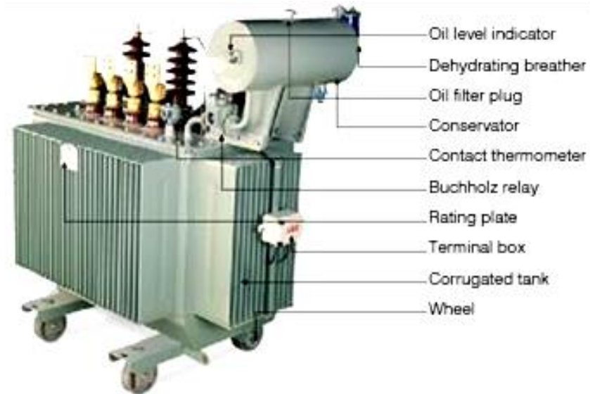
Figure 3.2 Transformer Structure
