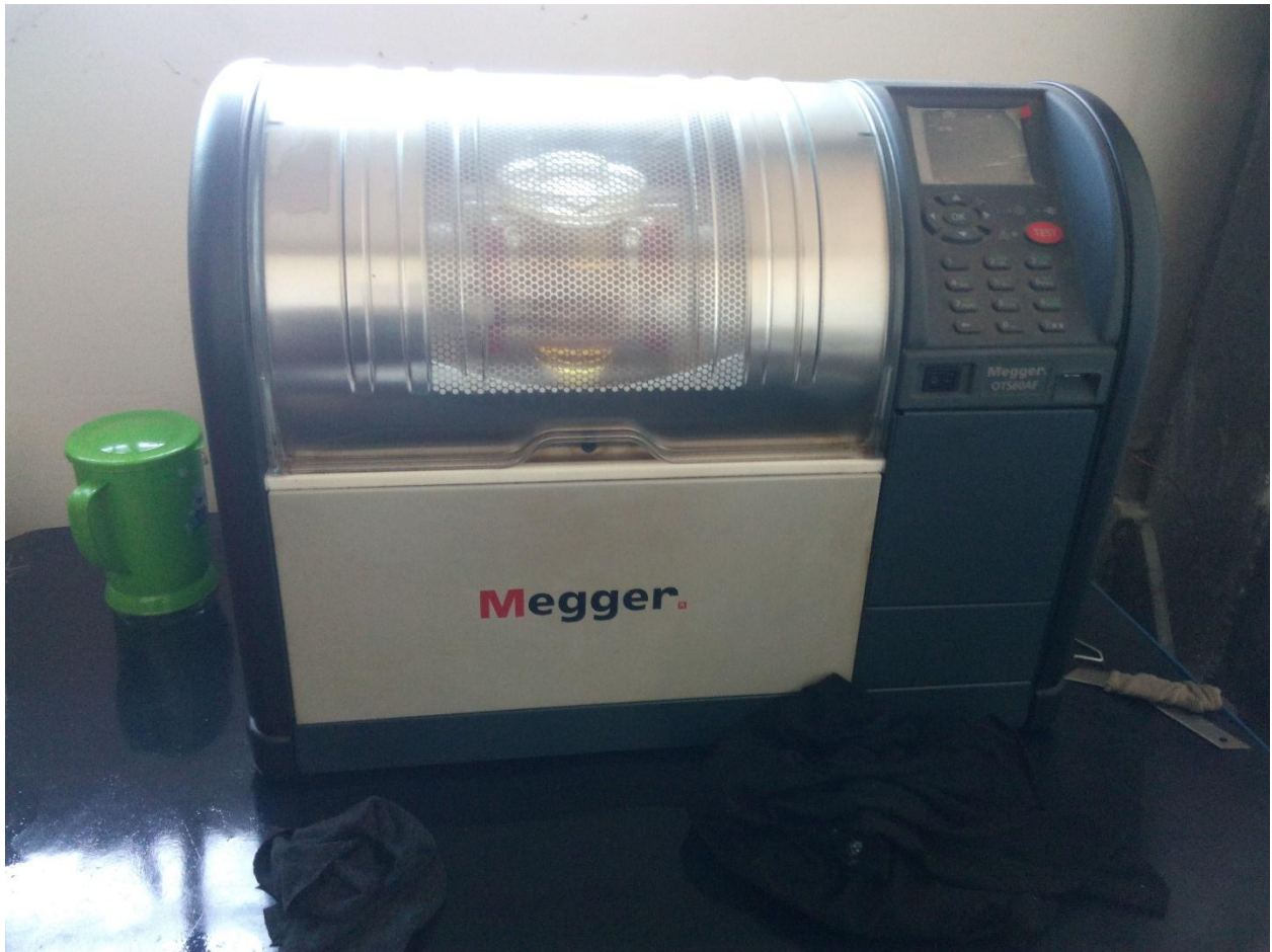
Fig. 2.8: Dielectric Oil Test Module of BREB-workshop
