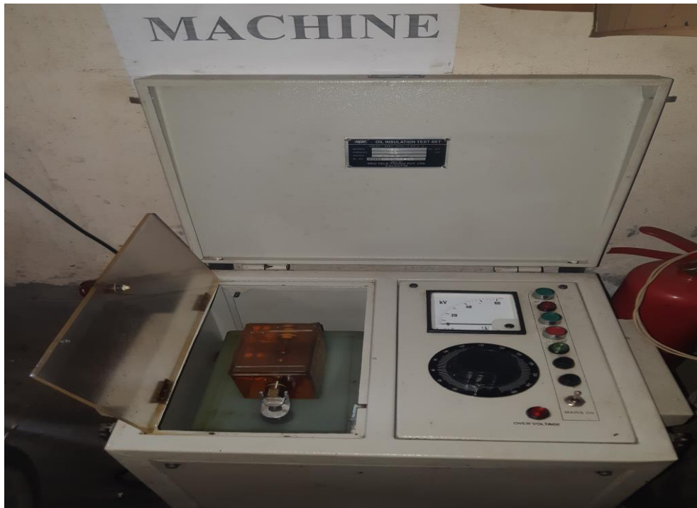
Figure 3.2: Transformer Oil Test Machine of Narayanganj PBS-1
