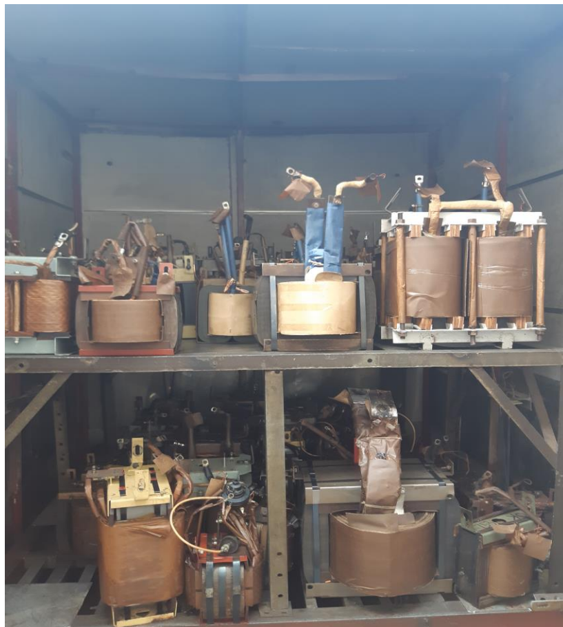
Figure 5.9: Heating Chamber of Transformer in Narayanganj PBS-1
