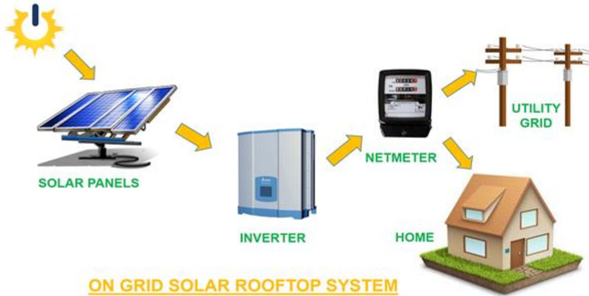
Figure-2.2: On grid solar rooftop system
