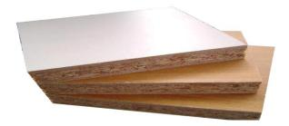
**Particle board**, also known as **particleboard** and **chipboard**, is an engineered wood product manufactured from wood chips, sawmill shavings, or even sawdust, and a synthetic resin or other suitable binder, which is pressed and extruded. Particleboard is a composite material.
