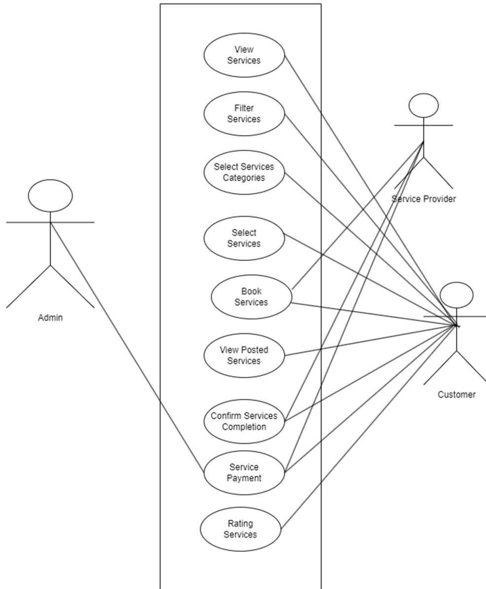
Figure 6: Use Case Diagram | Level 1.1, Shows the process from selecting a service to confirming a booking.
