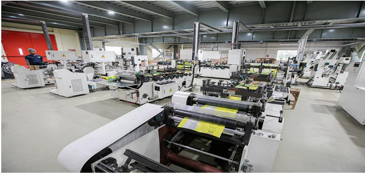
Figure-07: Slitting Machine of Arbab Pack Ltd.
