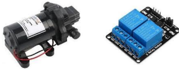
Figure 4.1-12: water pump and Relay
