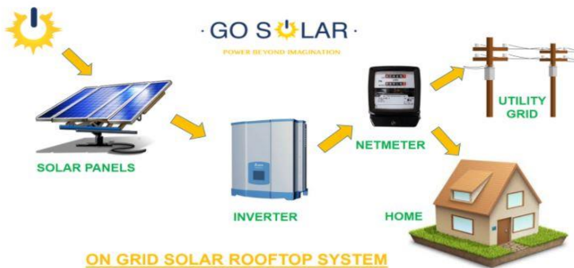
Figure: 2.10 On-Grid Solar Roof Top System
