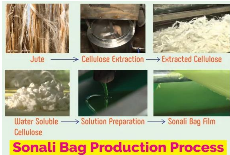
Figure 14: Sonali Bag Production Process
