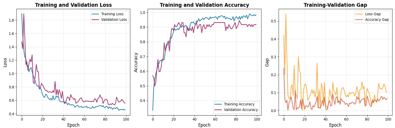
FIGURE 4.5: ResNet18 Training Curves (Loss, Accuracy, Overfitting Gap)
