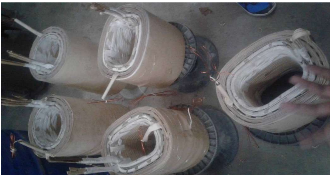
Figure: 3.15: Transformer winding
