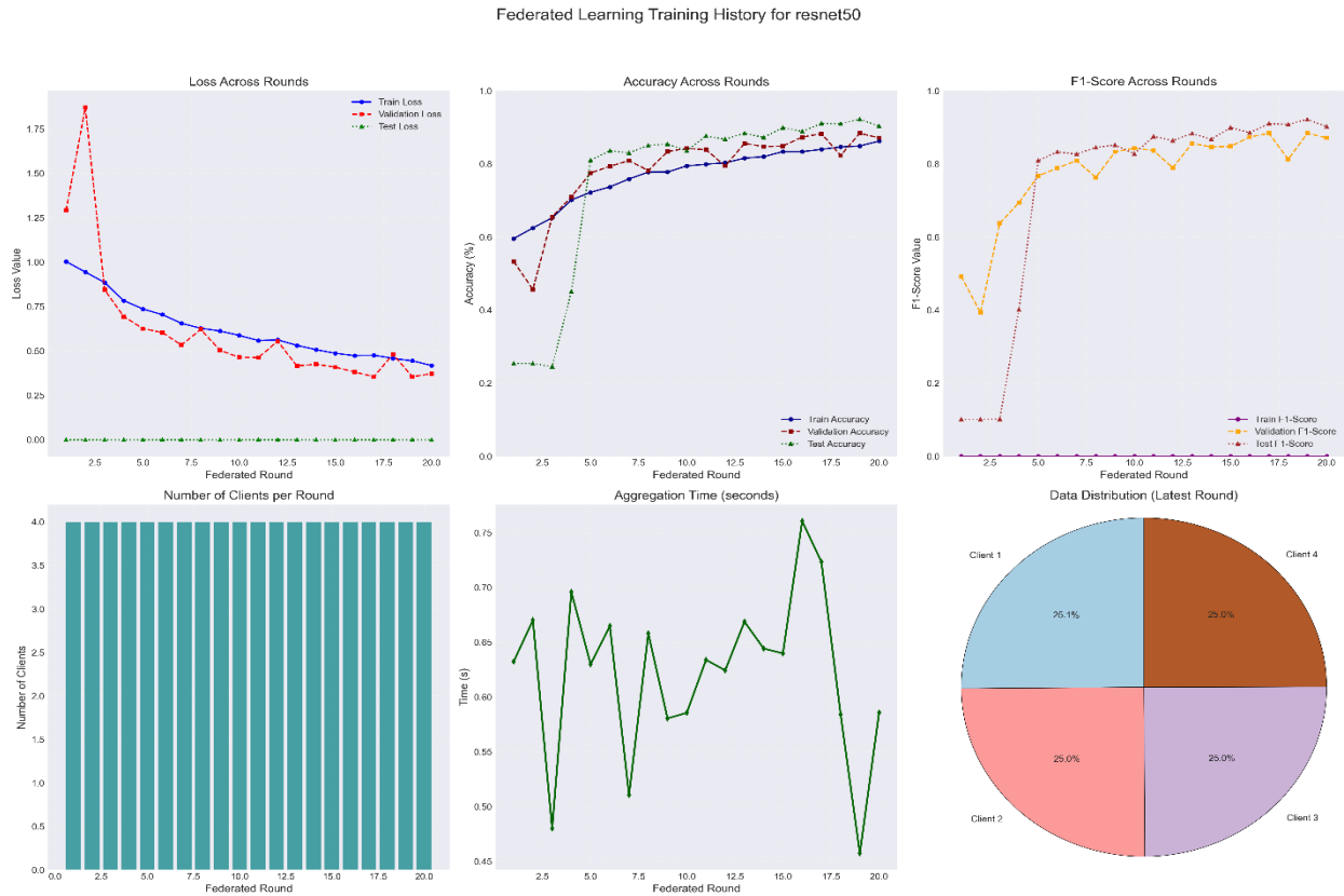
Figure 5: Federated training dynamics of ResNet-50: loss and accuracy curves, macro-F1, server-side aggregation time, and per-client data profiles across 20 FedAvg rounds (2 epochs/round).
