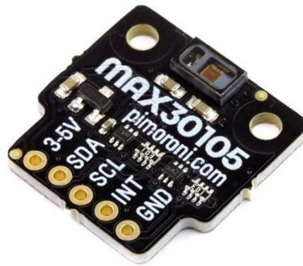
Figure 3.3.2: MAX30105 Pulse oximeter sensor module
