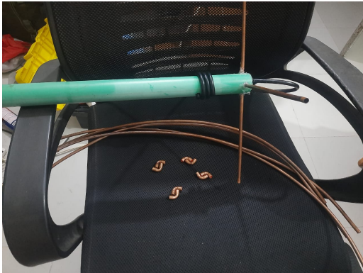
(a) Bending the QFH elements
