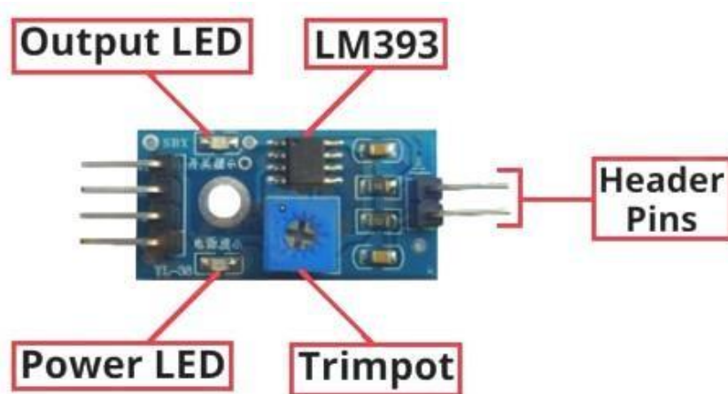
Figure 3.10.2: Identification and Explanation of Rain Sensor Pins
