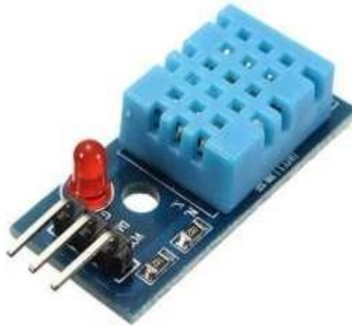
Figure 3.10: Humidity and Temperature sensor
