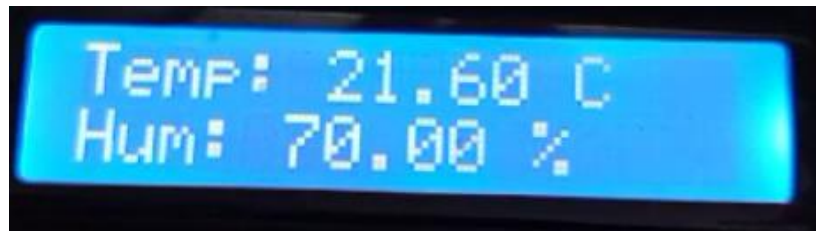
Figure 5.1: Temperature and Humidity Output
