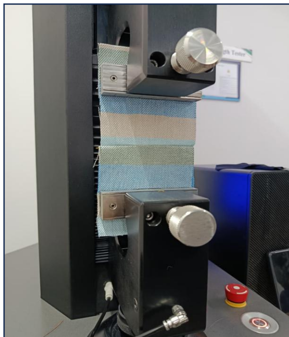
Figure 3.14 Herringbone weave before Tested
