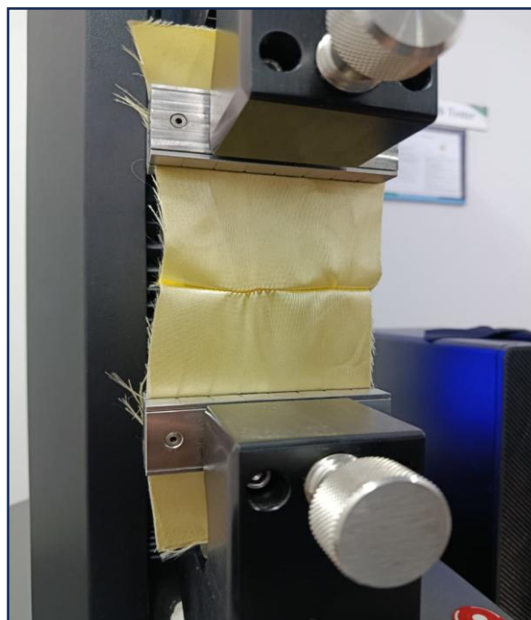
Figure 3.18 Satin weave Before Tested
