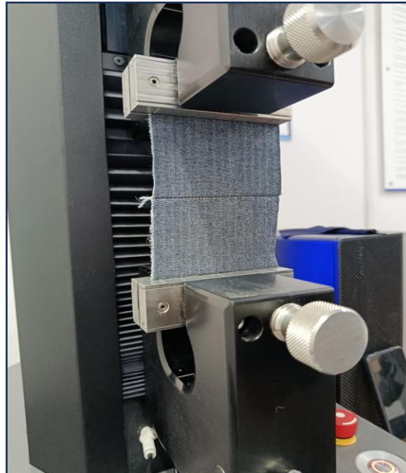
Figure 3.15 Zig-zag weave before Tested
