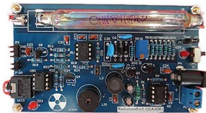
Fig. 4.2.1 Geiger-Müller (GM) Tube with High-Voltage Generator
