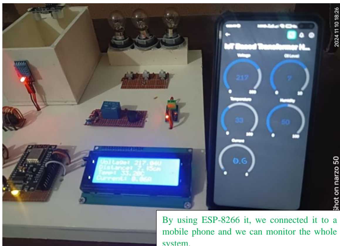
Fig:4.6 :IOT Based Monitoring System
