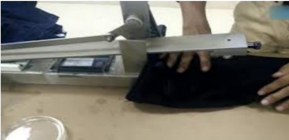
Figure 2.1: Rubbing fastness testing
