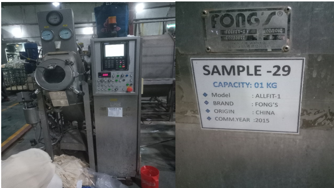
Figure 3.8: Sample Dyeing Machine
