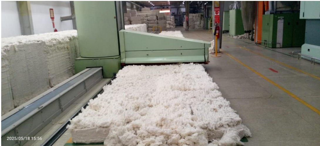
Blow Room Production rate (100%)=800 kg/hour Efficiency: 95%
