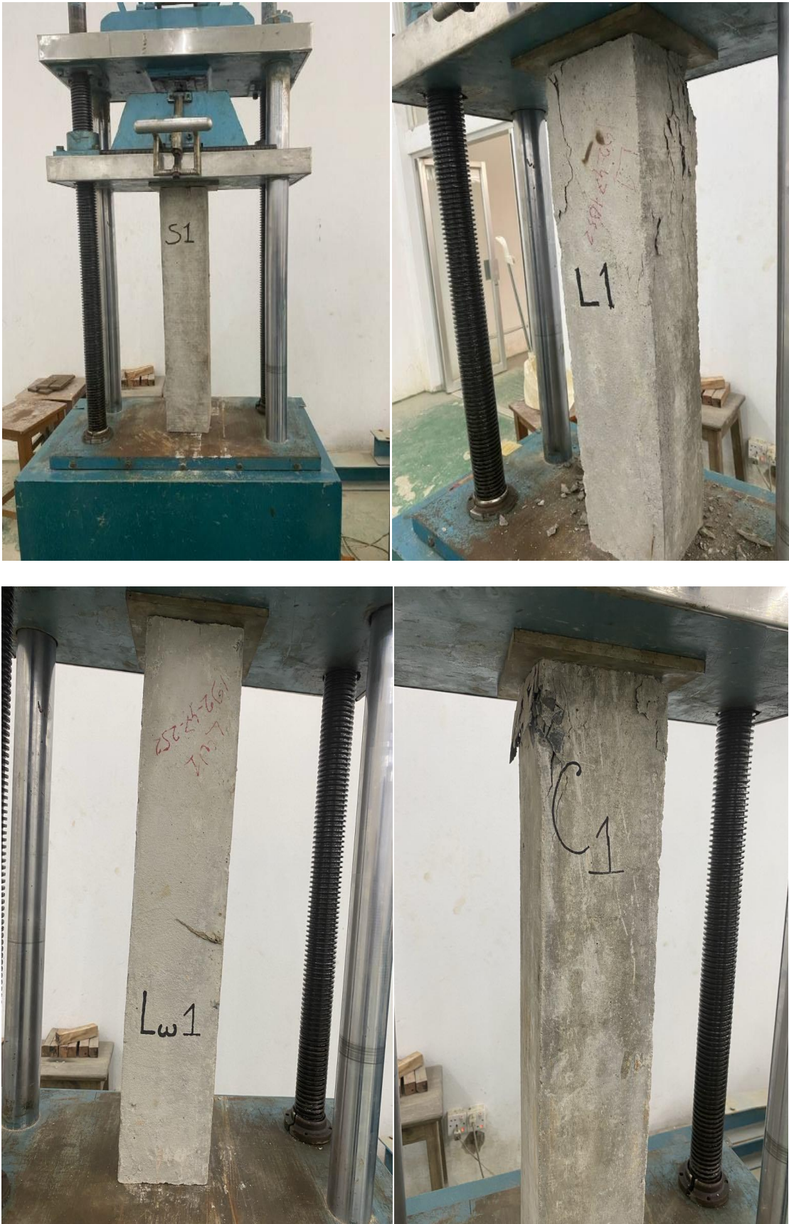
Figure 3. 6 Axial Load Capacity test of column in UTM
