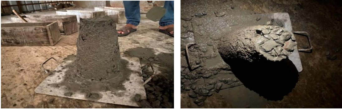
Figure 3. 4 Slump Test of Concrete
