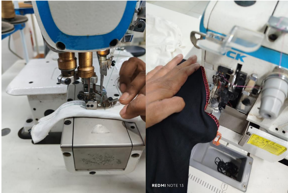
Figure 13: Flat lock with cover stitch
