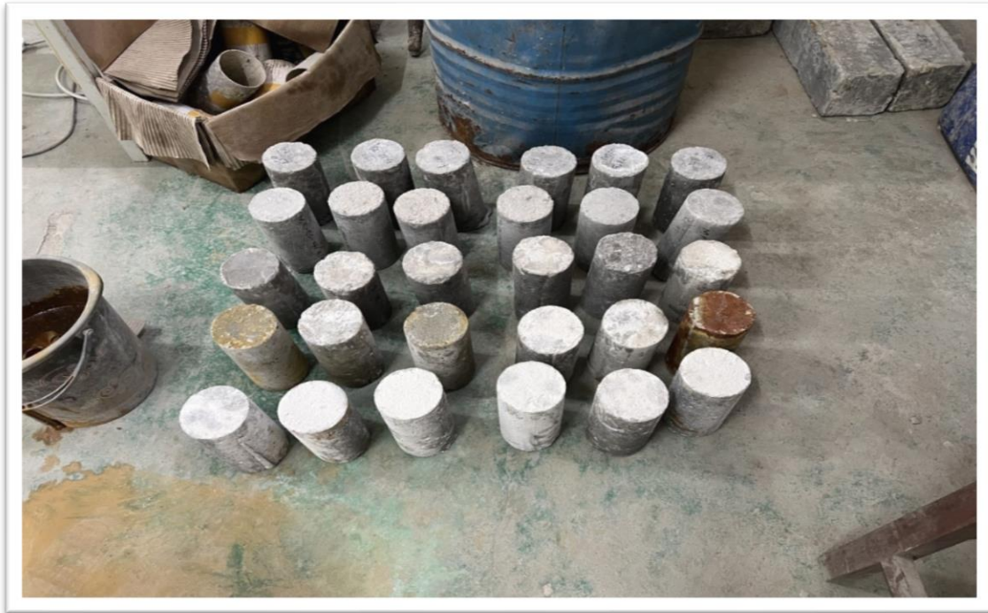
Figure 3.12: Specimen for the compressive & split tensile test
