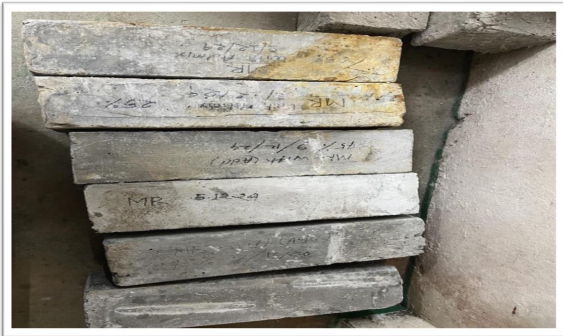
Figure 3.13: Specimen for the flexural strength test
