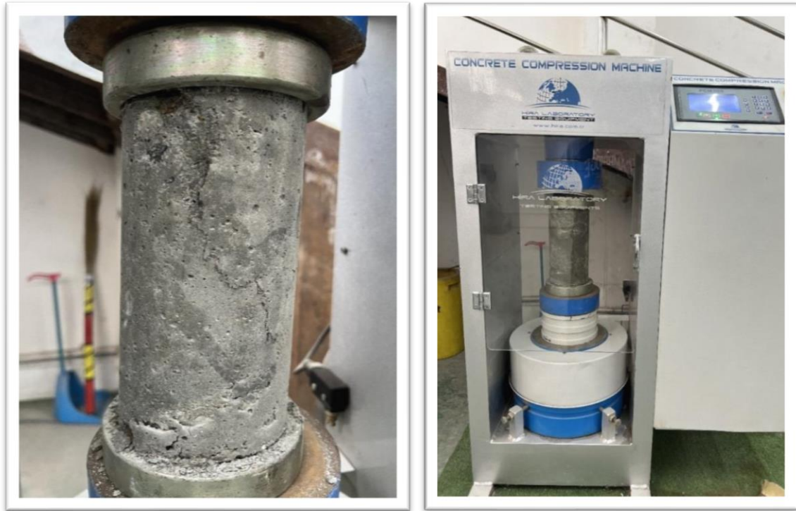
Figure 3.14: Compressive Strength Test.
