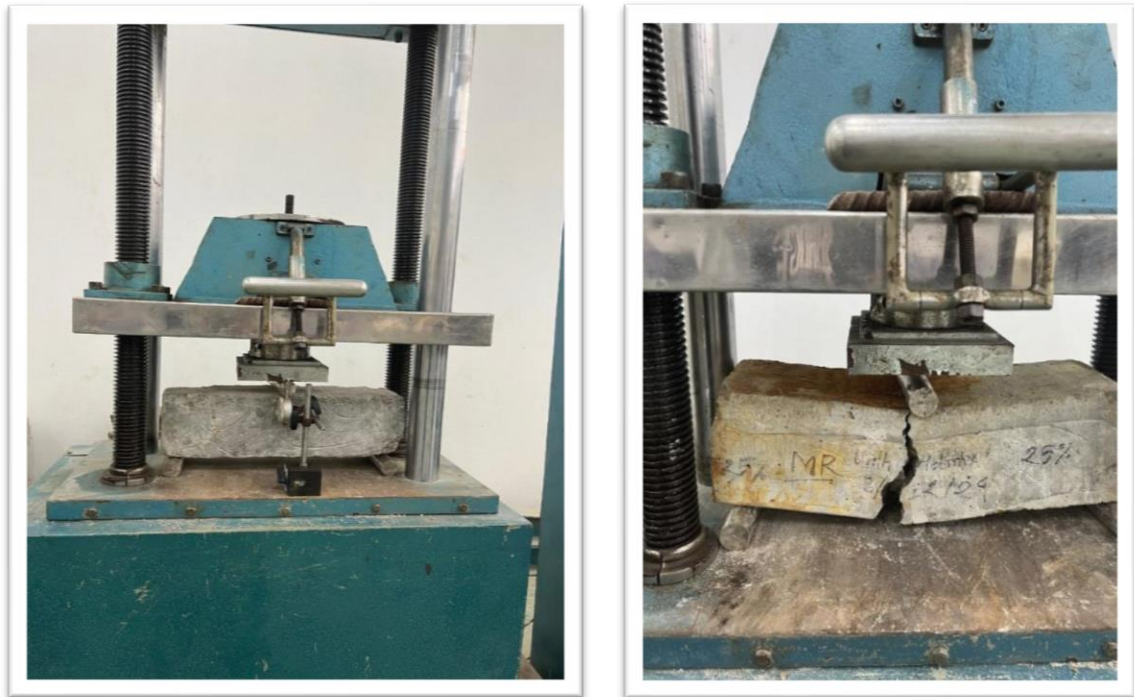
Figure 3.16: Flexural Strength Test
