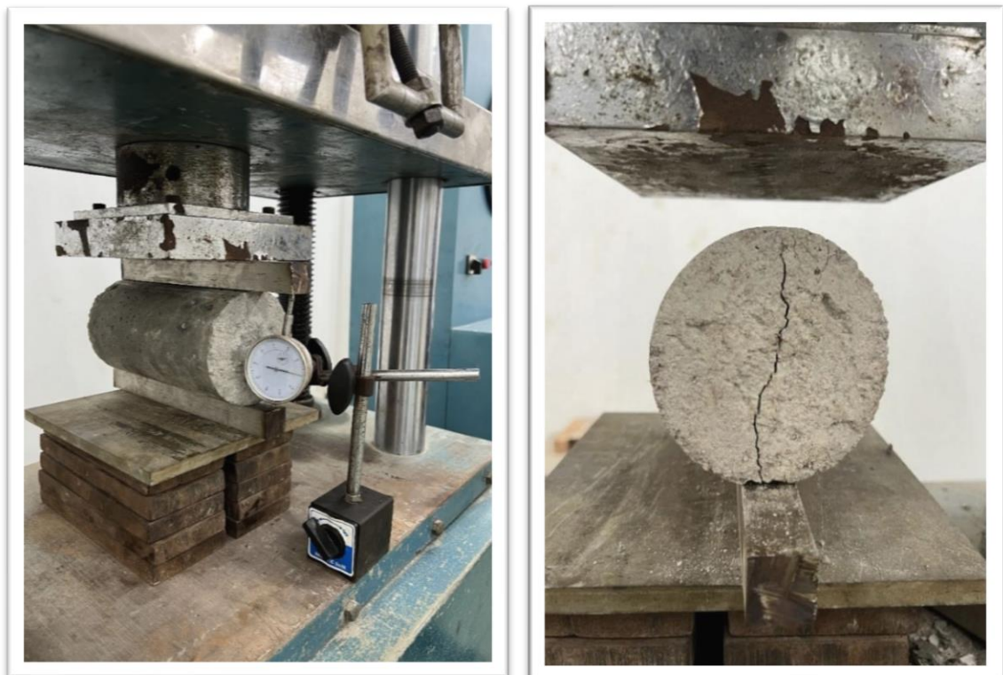
Figure 3.15: Split Tensile Strength Test
