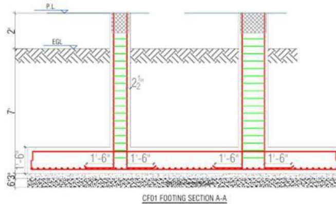
Figure 3.17: Typical CF-01 Footing (6'x13'), Thickness 15"
