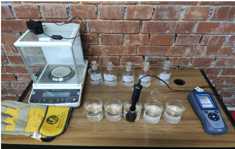
Figure 3.3: pH, DO, and Turbidity test Sample, detailed experimental procedure involving multiple instruments to analyze parameters such as pH, Turbidity, and Total Dissolved Solids (TDS)
