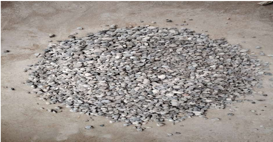
Figure 3.5 Demolition Coarse Aggregate
