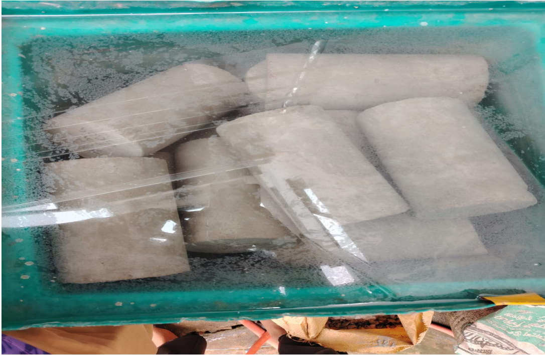
Figure 3.10 Curing of cylinder and beam
