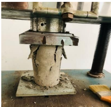
Figure 3.20 Compressive Strength Test of Mold
