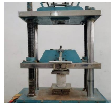
Figure 3.22 Compressive Strength at UTM
