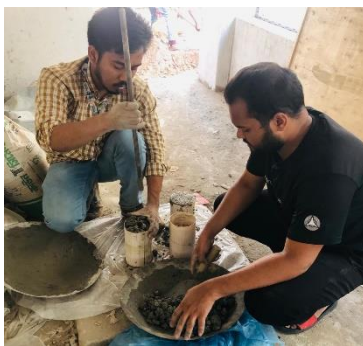
Figure 3.17 Compaction using Tamping Rod
