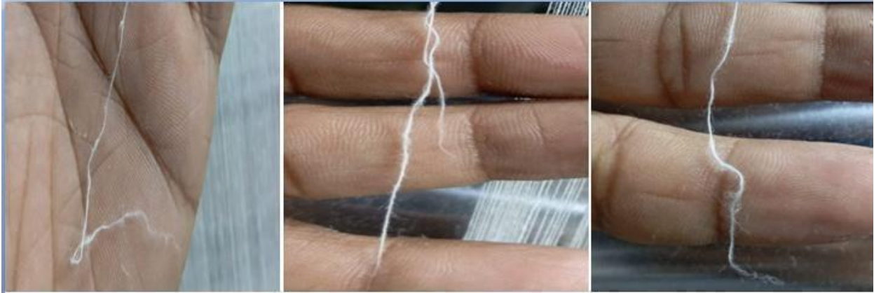
Figure: 4.11 A figure of fluffy warp yarn which is produced by friction between reed dent and warp yarn during the beating process.
