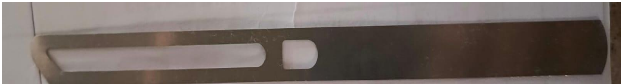
Figure: 2.17 Drop Wire bar
