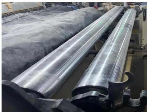
Figure: 2.31 Tension roller (Top) and backrest roller (bottom)
