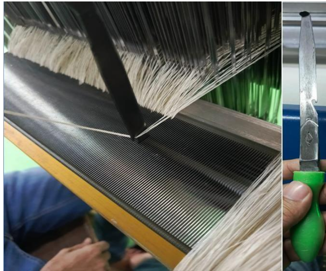
Figure: 2.9 Denting Process and Denting Hook.
