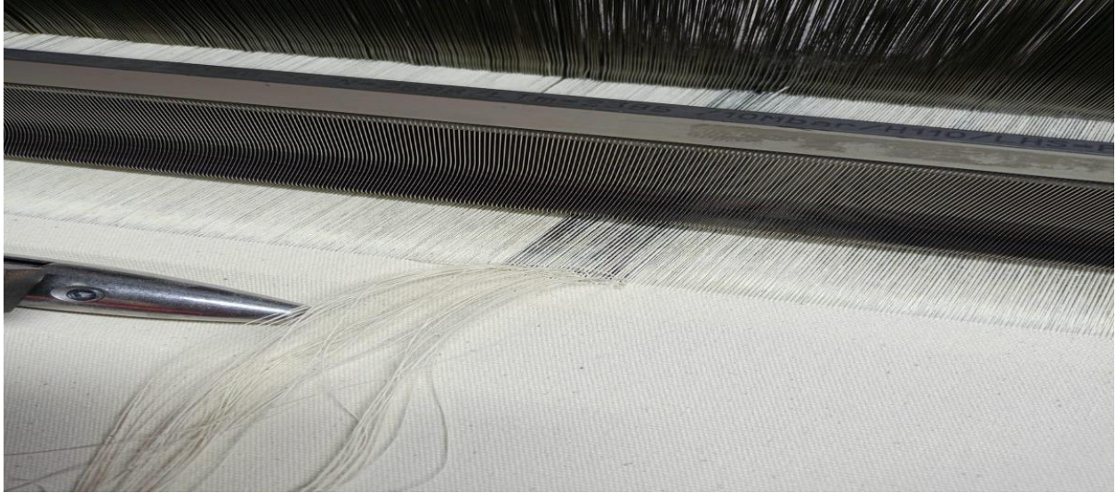
Figure: 4.4 Figure of warp yarn bunch breakage due to warping knots.
