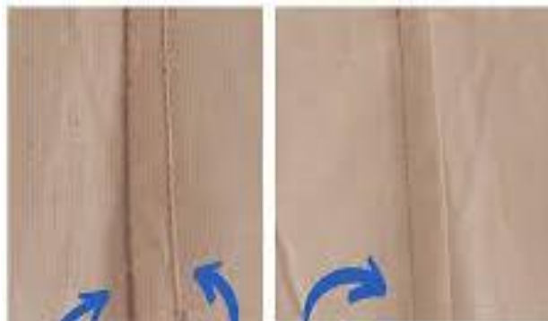
Figure 2.4: Incorrect Seam Line
