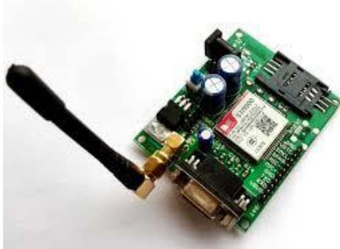
Fig 3.3: Typical GSM module
