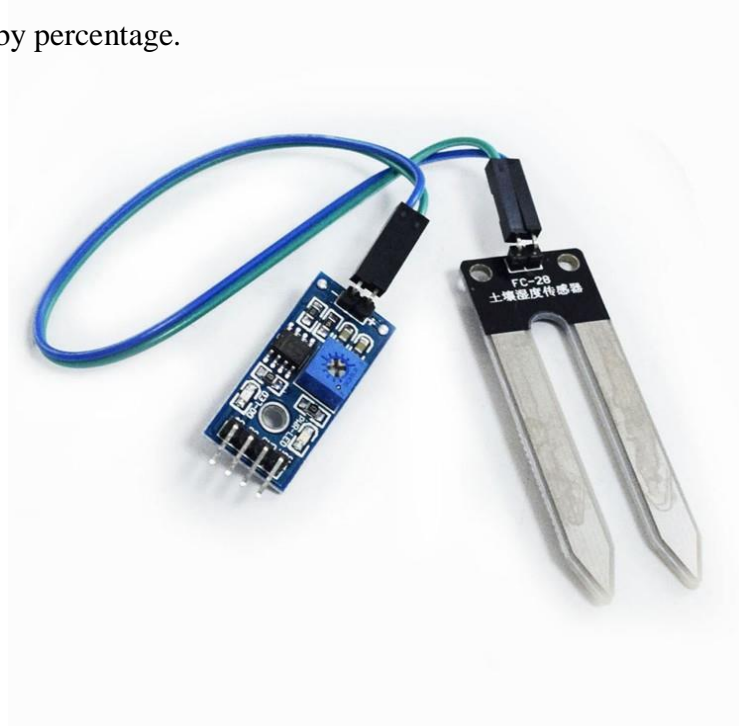
Figure: 3.8 Soil Moisture Sensors
