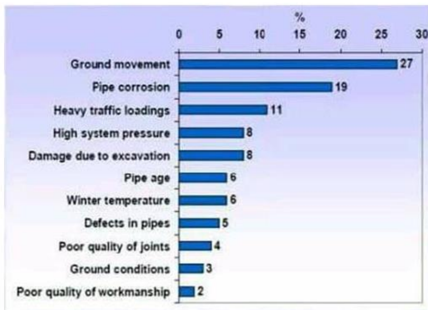
Figure 5.9 Percentages to the factors that causes leakage
