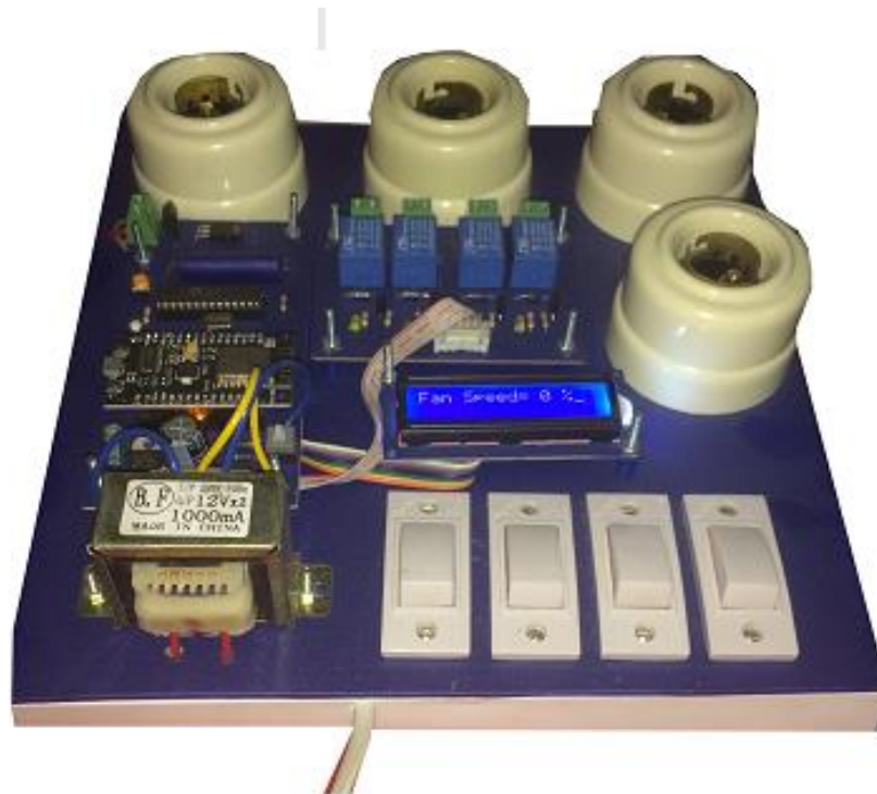
Fig: 2.7 IOT Based Home Load ON/OFF Switch with Fan Speed Controller
