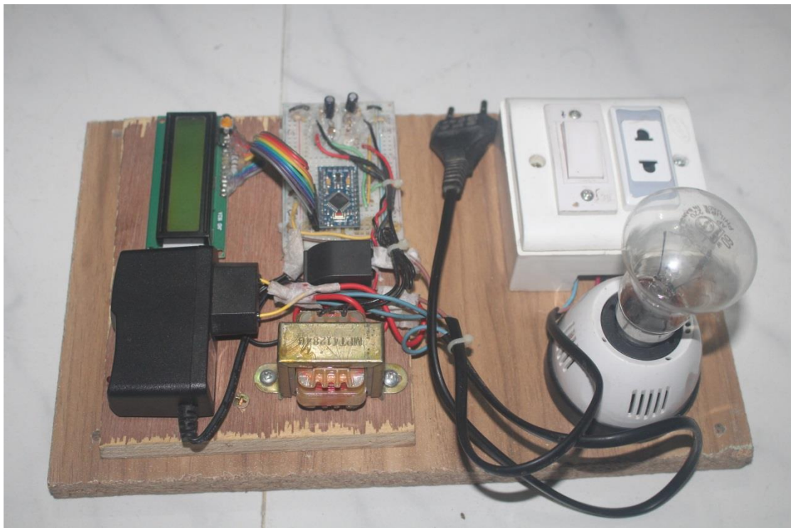
4.2: Photograph of design And implementation digital power factor meter
