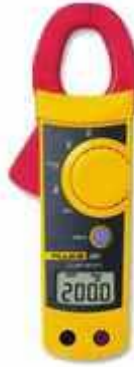
Fig 3.8.4: Handheld Current Transformers
