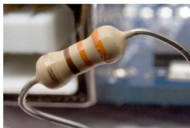
Fig 3.5: Resistor
