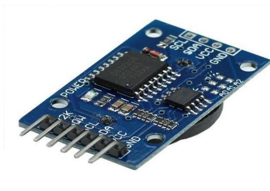
Fig 3.3: Real Time Clock (RTC)
