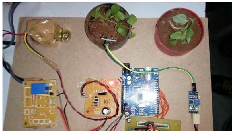
Fig. 2.3: complete circuit of automatic irrigation system
