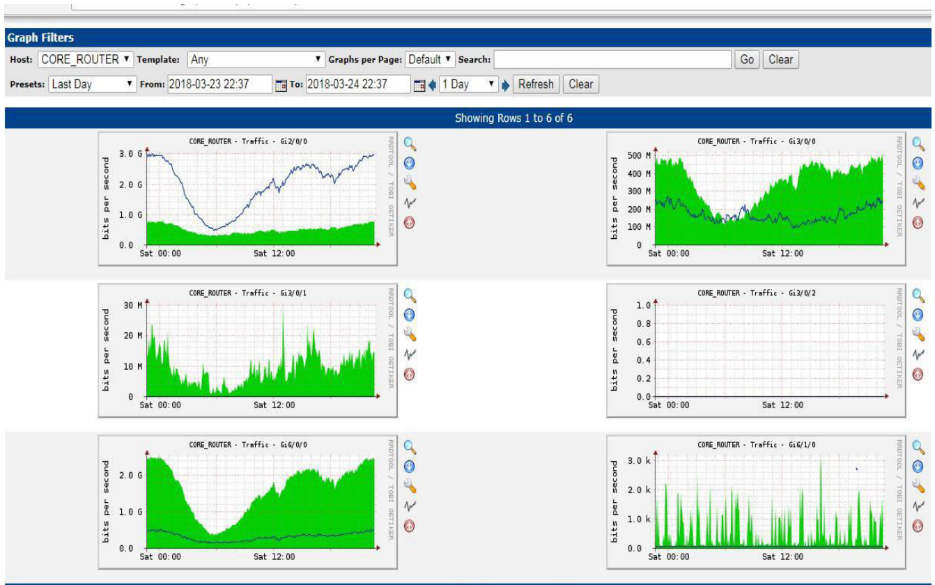
Figure 3.5: Traffic analysis for individual link showing on MRTG
