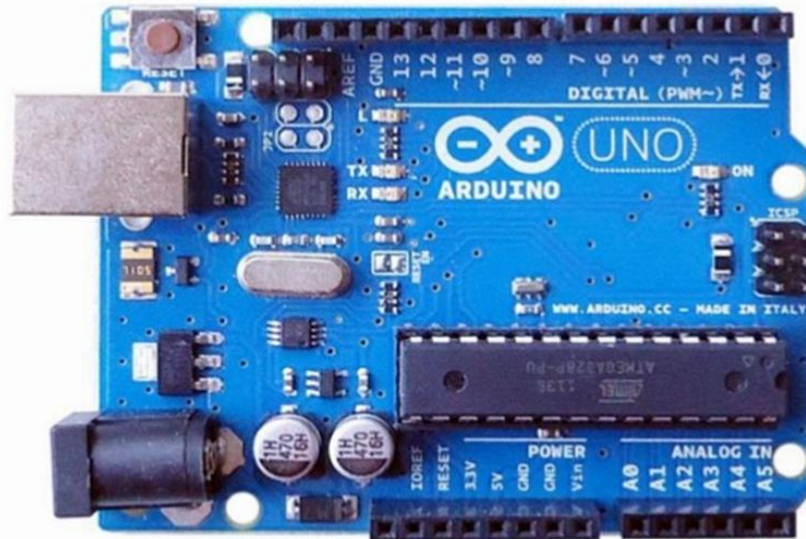
FIGURE 3.5: Arduino UNO R3 Board
