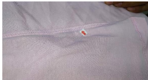
Figure: 2.8 Needle hole
