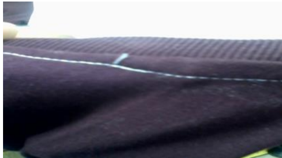
Figure: 2.4 Unbalance Stitch
