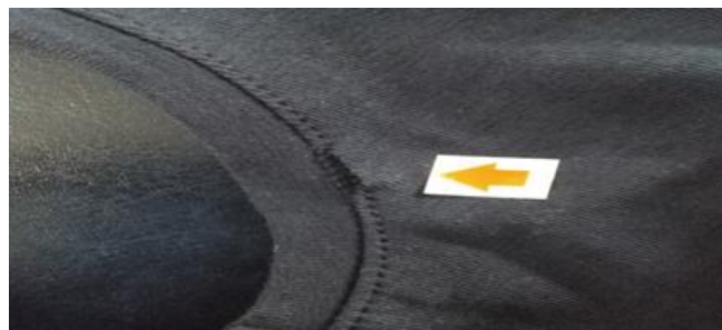
Figure: 2.5 Open Seam
