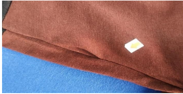
Figure: 2.2 Seam Puckering
