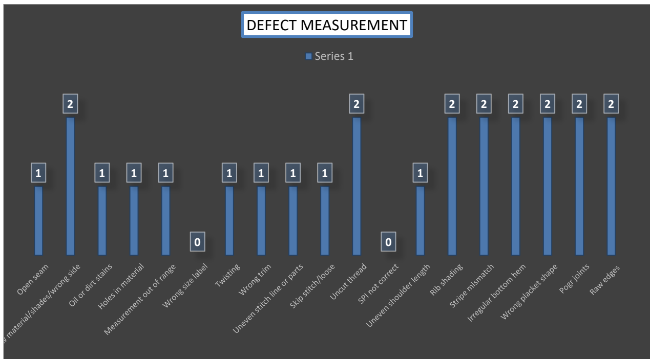
Figure: 4.1 Graphically Show Sewing Defects Number Measurement of In Line Operation Audit Report-1
