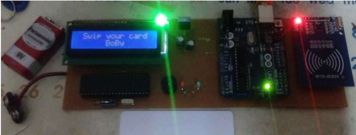
Fig 4.4: RFID based door lock with automatic door open and close
