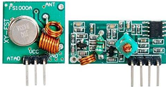
Fig 3.2.2: TX and RX module
